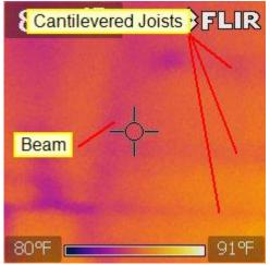
13.0 Picture 38 - Infrared photo of cantilevered joists
