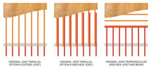
TYPICAL CANTILEVERED FLOOR CONSTRUCTION METHODS
